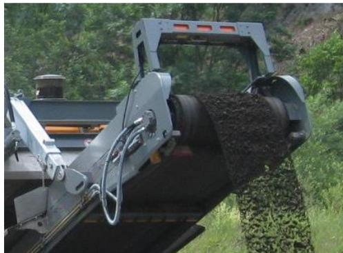
6. The **belt tension** plays a very large role at the conventional belt scales. It may change throughout the day due to temperature differences and cause incorrect measurements.
